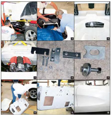
material needs to be removed, and marked the edge with masking tape. A vacuum can help keep the dust down considerably when cutting fiberglass and, as always, wear a mask and long sleeves when cutting fiberglass.
