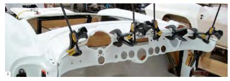
4 The removable dash panel (a benefit of Corvette Central's Concept '57 body) needed to be molded into position in preparation for painting. Again, you don't want to be doing any fabrication after the paint is applied.
