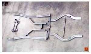
1. The most basic element of the chassis is the frame. Street Shop starts with .120-inch (approximately 1/8") walled 2X4" square tubing which is then mandrel bent to Street Shop's specifications. One of the problems on these cars is the rear section of the frame interfering with the underside of the body. Street Shop has extensive R&D in creating a frame with a minimum of interference between the body and frame.
